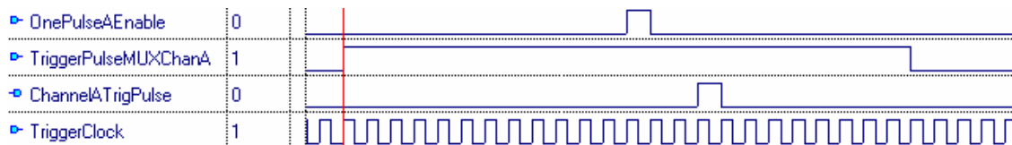
Figure 15. One pulse generated on trigger A output (ChannelATrigPulse).
